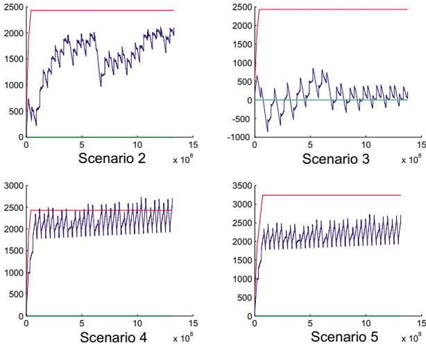
Fig. 5. Difference plots ( $x_{\max}(t) - x_{\min}(t)$  and  $x(t) - x_{\min}(t)$ ) for the simulation Scenarios 2–5, with the corresponding normalized buffer fill and emptiness levels of the playout buffer shown in Figure 6. The horizontal-axis shows time in ns and the vertical-axis shows the number of processed macroblocks in the playout buffer.
