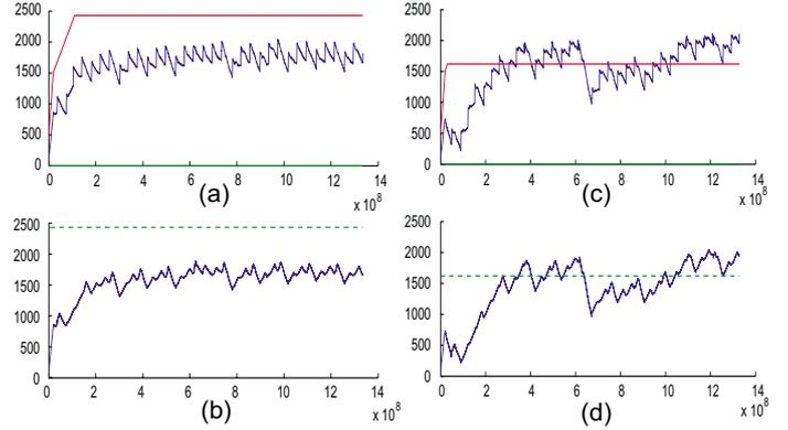
Fig. 4. (a) The difference plot for a macroblock stream  $x(t)$  which is compliant with the computed upper and lower bounds; (b) Corresponding playout buffer fill levels; (c) The difference plot for a non-compliant stream  $x(t)$ ; (d) Corresponding playout buffer fill levels indicating buffer overflow. The horizontal-axis shows time in ns and the vertical-axis shows the number of processed macroblocks in the playout buffer.
